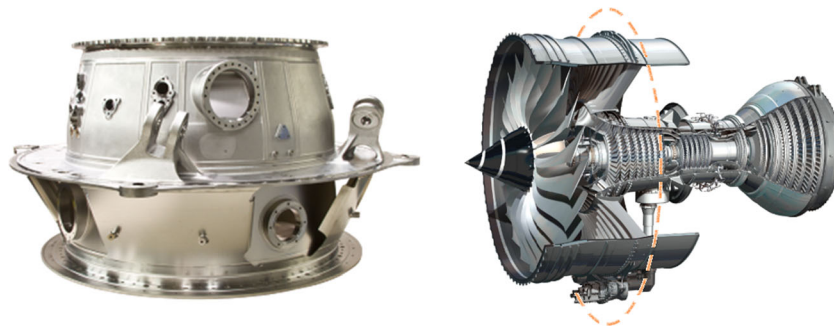
Fig. 1 The left picture shows a TRENT XWB-ICC (intermediate compressor casing). This fabricated ICC contains two different titanium alloys and is made from several different material forms (sheet, cast,
