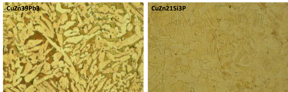
Fig. 1 Optical micrograph on the structure of the evaluated materials. CuZn39Pb3 (left) and CuZn21Si3P (right)
