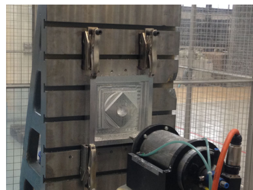
Fig. 2 Robotic machining set-up with work-piece mounted on the fixture with finger clamps
