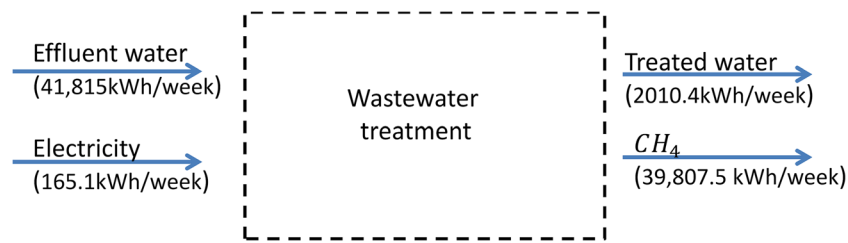
Fig. 3 Weekly averaged exergy flows through a typical AD process employed to hypothetically treat the food factory effluent
