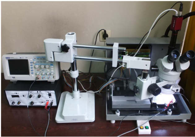
Fig. 1 Experimental setup (RC generator on the left)
