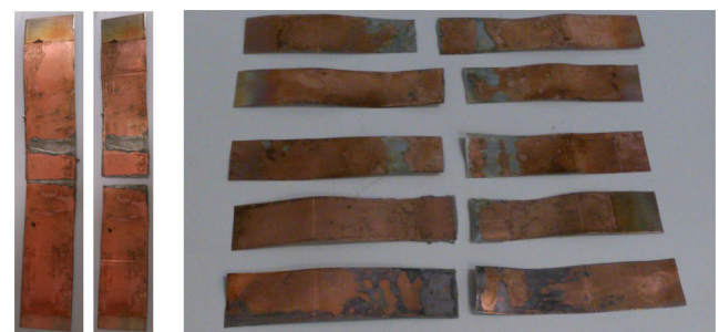
Fig. 6 Failure modes of copper lap-shear specimens
