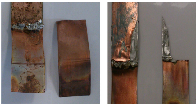
Fig. 8 Fracture modes of copper peel test
