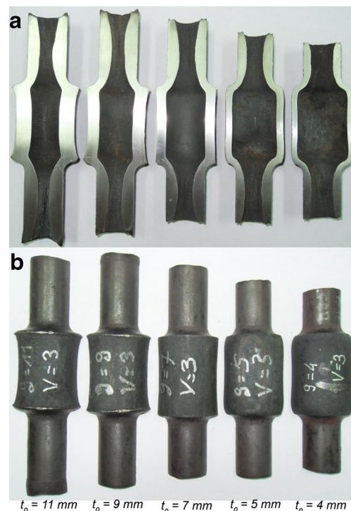
Fig. 11 Shafts produced by rotary compression in the experimental tests: a axial section and b general view
