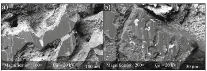
Grinding parameters:  $v_s$ =60 m/s;  $v_w$ =1.5 m/s;  $a_e$ =0.20 mm;  $v_{ja}$ =10 mm/s;  $v_{jr}$ =0.2 mm/min;  $Q_c$ =4.0 l/min; Grinding wheel: 1-35×10×10-SG/F46G10VTO | Workpiece: bearing rings made of 100Cr6 steel (62±2 HRC) Coolant: 5% water solution of Castrol Syntilo RHS oil given by flood method Surface condition: after grinding of 100 workpieces ( $V_w$ =46,400 mm<sup>3</sup>)
