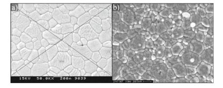
Fig. 17 Microscopic view of the nanocrystalline sintered corundum microstructure:
