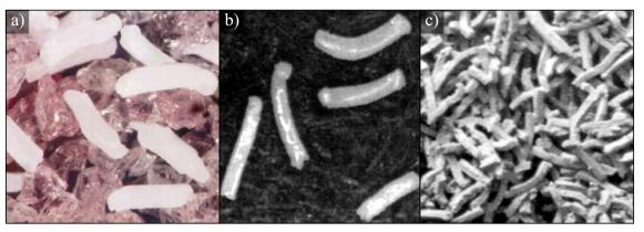
Fig. 15 View of the microcrystalline sintered corundum grains with elongate shape: a TG<sup>TM</sup> grains with dimension proportion 4:1 mixed with CrA grains; b TG2<sup>TM</sup> grains with shape proportion 8:1; c Norton's Altos<sup>TM</sup> wheel structure with TG2<sup>TM</sup> grains [49, 50]
