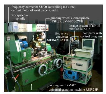
Fig. 11 General view of the experimental setup
