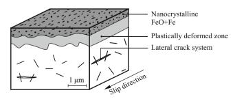
Fig. 10 Schematic illustration of the structure of the smoothed surface of microcrystalline sintered corundum [40]
