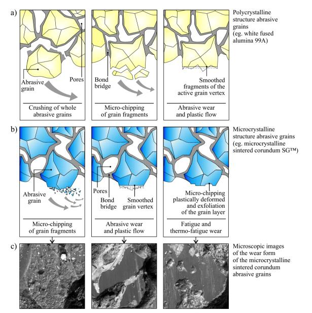
Fig. 14 Grain breakdown models in grinding wheels with polycrystalline (a) and microcrystalline (b, c) alumina abrasives (based upon drawings of the Rappold Winterthur Group and the author's own materials)
