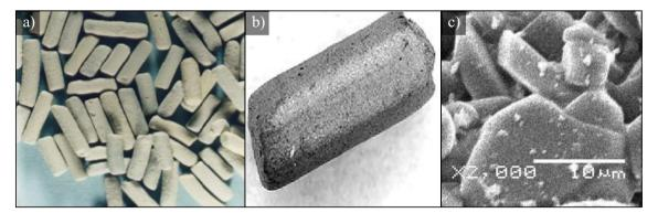
Fig. 4 Zirconic sintered corundum abrasive grains: a overall view—magnification×4; b abrasive grain magnitude×40; c microstructure of the abrasive grain—magnification×2,000 [24]
