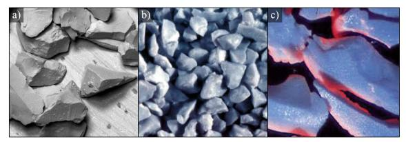
Fig. 7 View of the microcrystalline sintered corundum grains: a SG<sup>TM</sup> grains—magnification×100; b Cubitron  $321^{TM}$ —magnification×50 [16]; c Sapphire Blue<sup>TM</sup> grains—magnification approx. ×500 [21]
