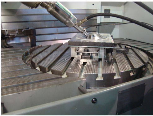
Fig. 1 Normal position of hydraulic burnishing tool with integrated force gauge during 3D surface machining on five-axis machining center DMG DMU 60 MONOBLOCK [2]
