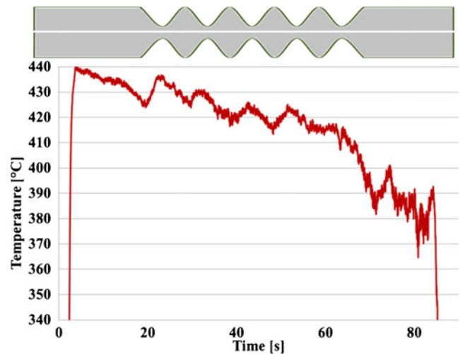
Fig. 12 Temperature signal for the sinusoidal shaped workpiece without controller. The geometrical shape of the workpiece (top) is mapped with the time plot to indicate the locations corresponding to the temperature peaks
