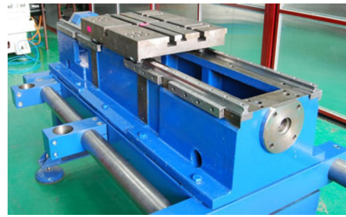
Fig. 10 The view of the stand for the milling table examination
