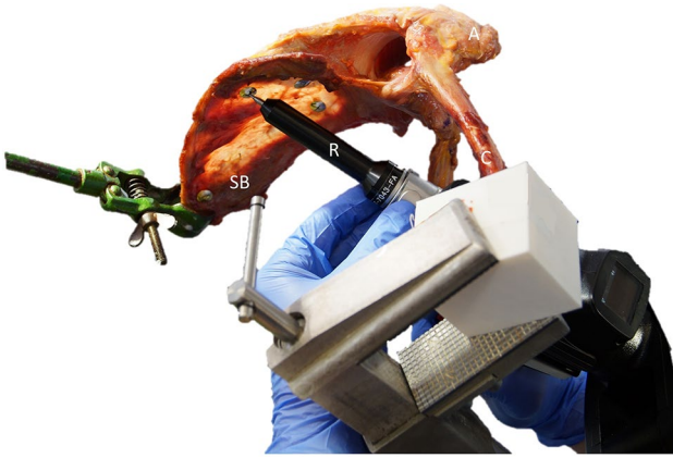
Fig. 1 Fixation of the scapula (SB) and clavicle (C) during initial measurements of anatomical ligamentous insertions and reference pins for the definition of a rigid body system. (R Romer arm, A Acromion)
