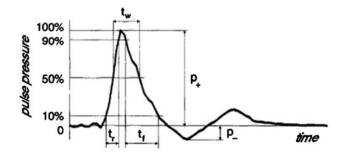
Fig. 1 Pressure-time profile of a shockwave (reprinted from [6])
