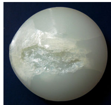
Fig. 5 Retrieved patellar component showing signs of catastrophic wear characterised by a variety of wear mechanisms including cold flow, pitting, abrasion, sub-surface fracture, and delamination
