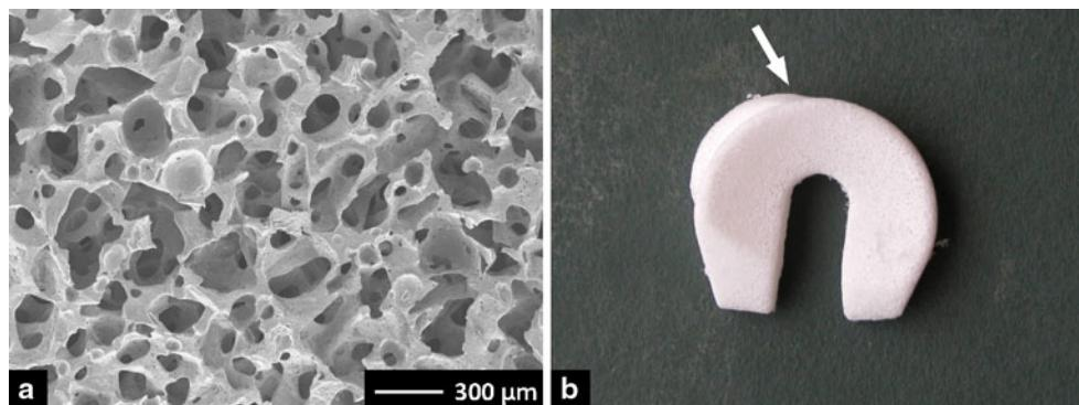
**Fig. 1** **a** Scanning electron microscopy image of a cross section of the polycaprolactone-based polyurethane (PCLPU) implant. **b** Porous PCLPU meniscus implant provided with an interstice for the popliteus tendon (arrow)
