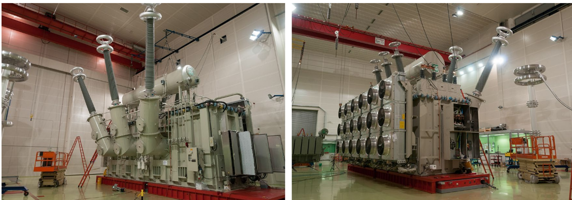
Fig. 5 An example of two power transformers, where the same functionality is realized with two very different shape models. Agile PD plays a key role in company competitiveness
