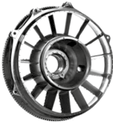
Fig. 1 Example of a complex jet engine component embodying many functions and can be fully casted as one single piece (GKN Aerospace 2014)
