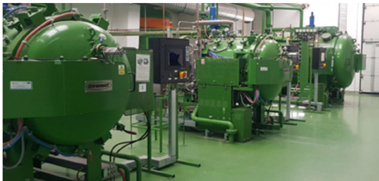
Fig. 4 Sintering of tungsten rods in a chamber furnace
