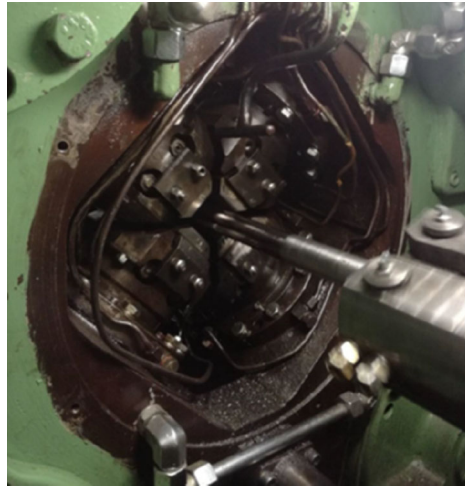
Fig. 5 Cold swaging rods on a radial swaging machine STEYER SPH06.09
