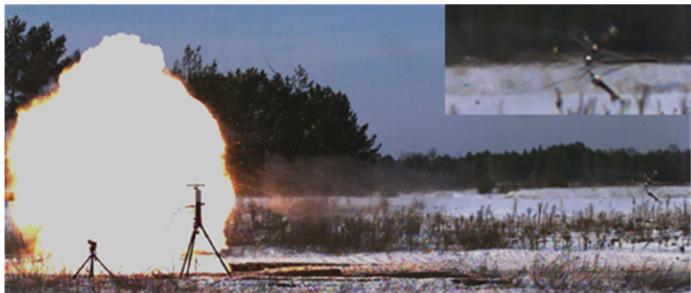
Fig. 12 A frame from firing a round conditioned at temperature of 233 K
