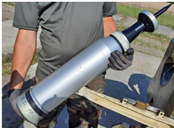
Fig. 10 120 mm sub-caliber projectiles with new WHA penetrator before loading to gun
