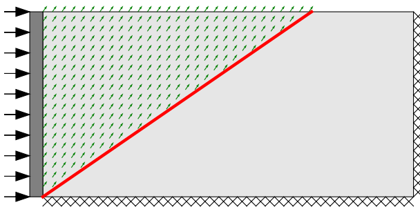
Fig. 14 Retaining wall: DLO solution for 40 \times 20 nodal division case, \lambda = 23.254 (smooth wall subject to unit load and taking c = 1, \phi = 20^\circ, \gamma = 1 )
