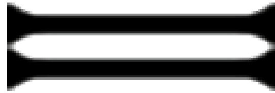
Fig. 17 Optimised design of uniaxially loaded Cauchy plate with central crack reported for a filter radius of r_{\min} = 0.04L considering Heaviside projection method (HPM)
