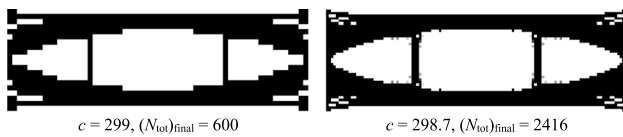
Fig. 16 Optimised design of uniaxially loaded Eringen’s plates without filtering
