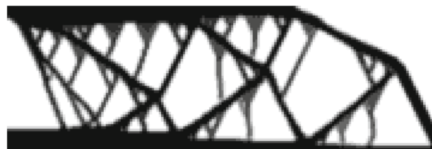
Fig. 6 The same problem as in the lower picture of Fig. 5, except that the maximum overhang angle is changed from 46^\circ to 30^\circ . The relative optimal compliance C = 1.13
