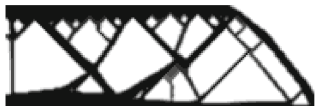
Fig. 4 The MBB beam using Langelaar’s AM filter, C = 1.11 . Note the sharp corners where overhang constrained boundaries meet
