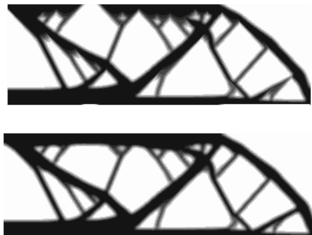
Fig. 9 Comparison of the overhang free design \rho^{of} in the upper picture and the corresponding physical design \rho in the lower picture
