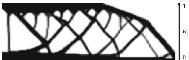
Fig. 8 The MBB beam using the penalty approach with p = 1 , q = 0.5 , \gamma = 10^{-5} and weights defined in (10). The build direction is shown by an arrow. The corresponding relative optimal compliance C = 1.10
