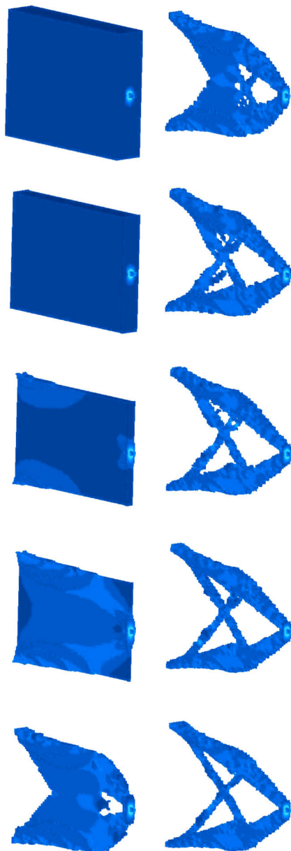
Fig. 3 Optimization results of the cantilever beam bending using of the biomimetic procedure, based on the trabecular bone surface adaptation - standard topology optimization domain full of material
