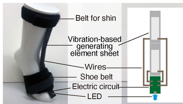
Fig. 1 System design of Ankle-Worn Sensor Sleeve, LED version
