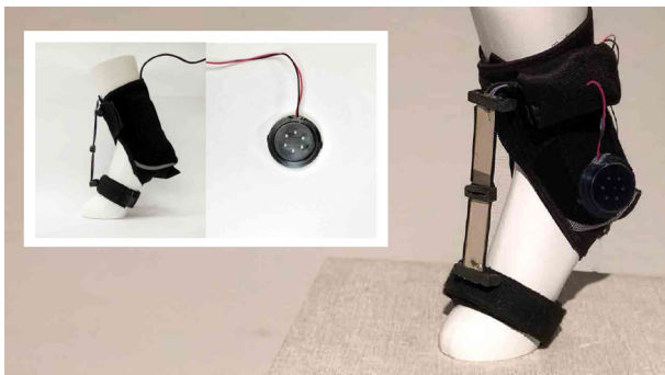
Fig. 6 Vibration feedback system
