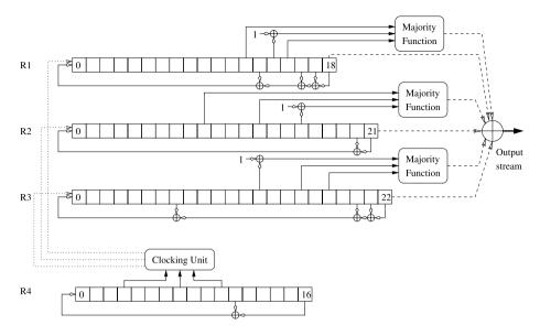
**Fig. 1.** The internal structure of A5/2.
