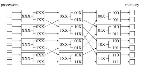
Fig. 1. Switching network connecting processors to memory.
