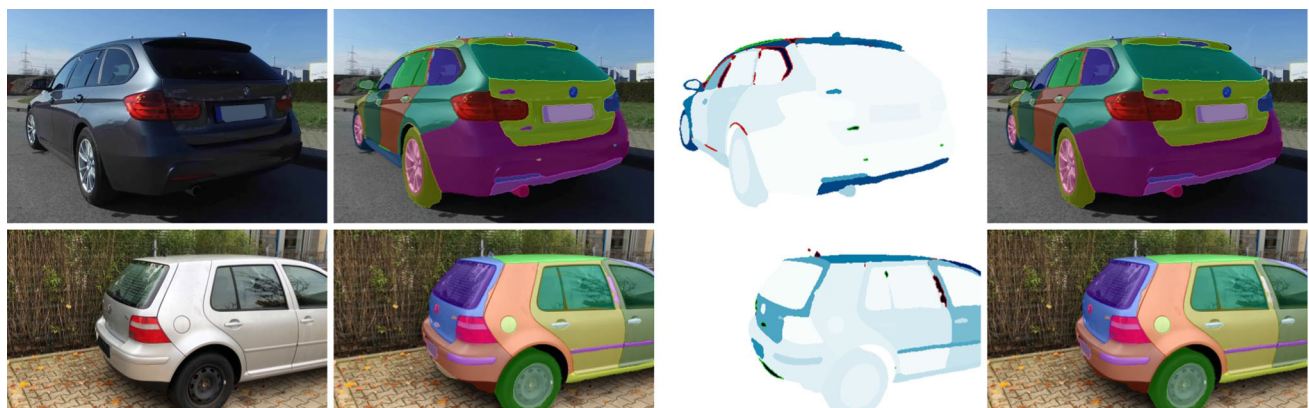
Fig. 9 Additional examples, showing (from left to right) the original image, the segmentation mask, the heat-map of the segment-wise uncertainties and the corrected segmentation mask. Several mistakes, for example on the rear bumper in the upper image and on the trunk in the lower image, are removed
