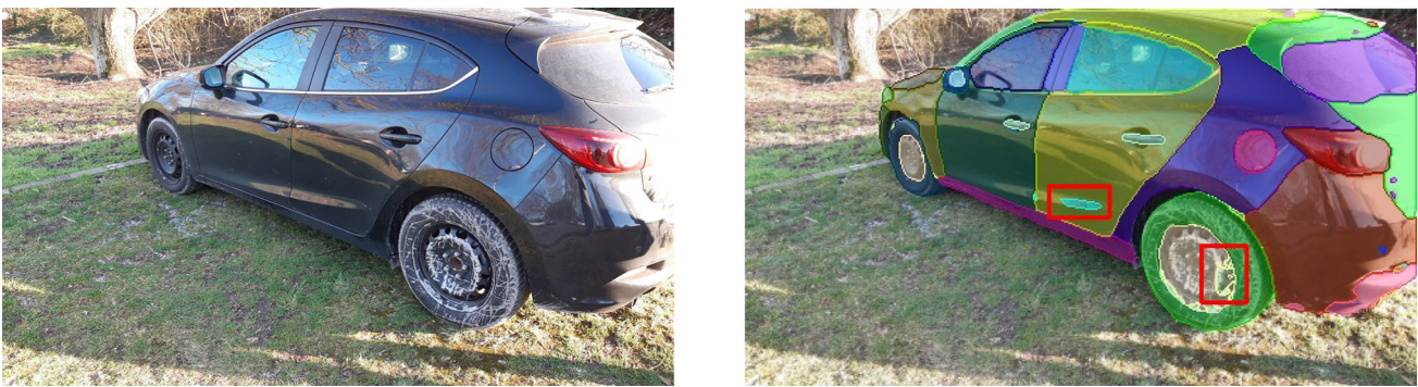
Fig. 1 Photograph of a car (left), taken to highlight issues that can negatively affect the performance of DNN segmentation models: reflections, dirt and bad exposure. Result of our semantic segmentation model (right), trained to segment car body parts. Predicted segments are shown
