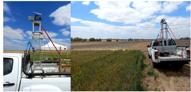
Fig. 5 Test dataset creation experiment at Gilat Research Center. The unique structure of the HS system was designed to be placed on a stand in a pickup truck to shoot the scene
