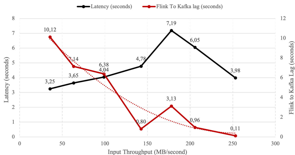
Fig. 17 Video2Flink speed-up and Flink to Kafka lag for parallelization 8 and YUV video
