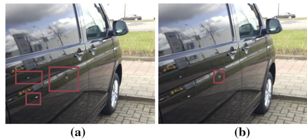
Fig. 7 Excerpt of a modified class label with iteration 1 (a) and iteration 2 (b). 2 removed false positives and 1 revised bounding box dimension
