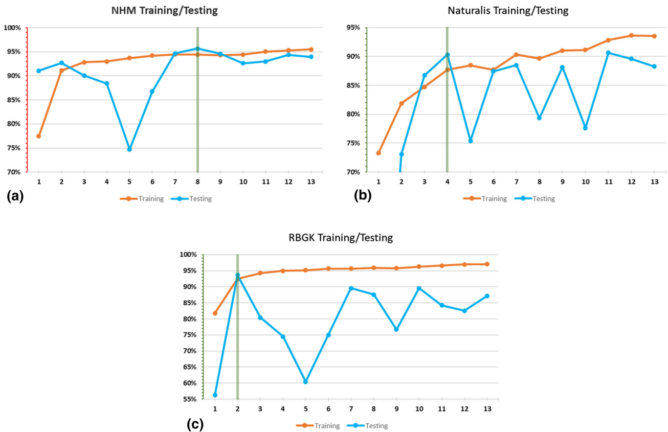
Fig. 7 Graphical view of the identification of the peak learned models for the microscope slides datasets: a NHM, b Naturalis and c RBGK. The orange line indicates the testing accuracies, which improves constantly as learning progresses, while the blue line marks the results of segmenting the test set. The green vertical indicates the epoch corresponding to the model selected for cross-validation
