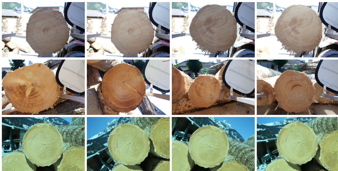
Fig. 6 1st Row ( TS_1 ): Respectively, two CS-Images from two different logs—one captured with flash and one without flash. 2nd Row ( TS_2 ): Four CS-Images from different logs. 3rd Row ( TS_3 ): Four CS-Images illustrating the rotational variations
