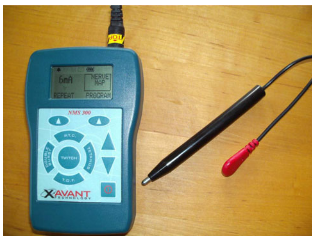
Fig. 1 Nerve stimulator (Xavant NMS 300) with nerve mapping electrode
