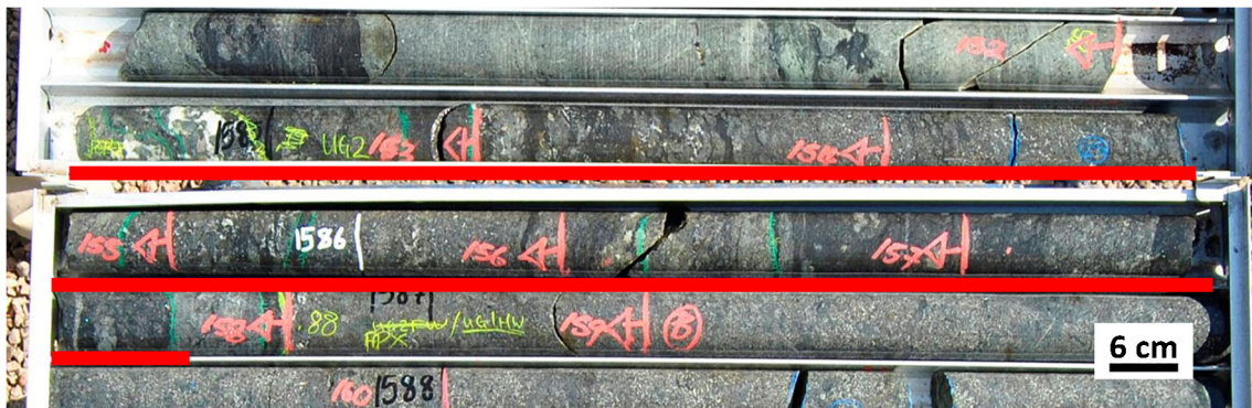
Fig. 2 The UG-2E chromitite seam interval in drill-hole UMT366 is indicated by the red underline. The hanging wall consists of feldspathic pyroxenite; dark sections are parapyroxenite (assimilated material). The UG-2E chromitite seam is intersected at a depth of 1584.88 to 1586.77 m (approx. 189-cm-thick); it is comprised of massive to semi-massive
