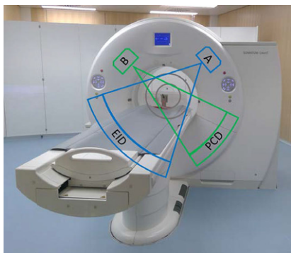
Fig. 4 ▲ The SOMATOM CounT computed tomography (CT) system at the German Cancer Research Center (DKFZ). The position of the energy integrating detector (EID) and photon-counting detector (PCD) and the corresponding two X-ray sources A and B are marked in blue and green. The housing is identical to a conventional clinical CT system
