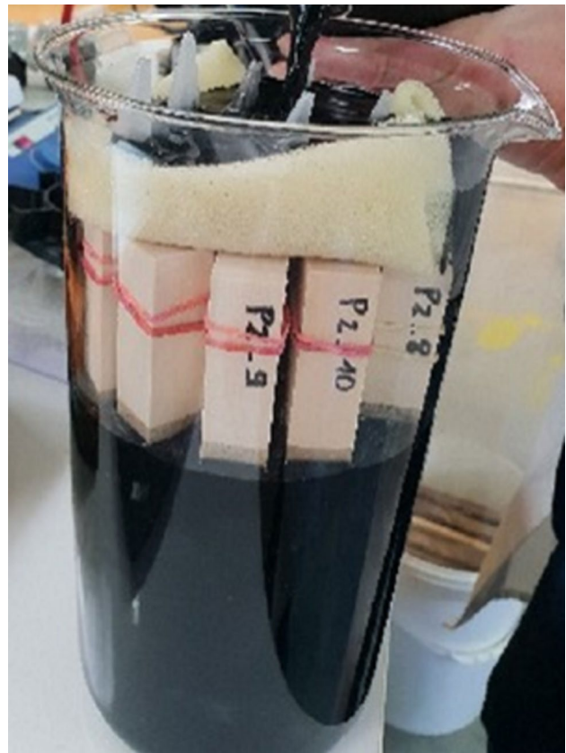
Fig. 1 Immersion of specimens in biochar + water mixture
