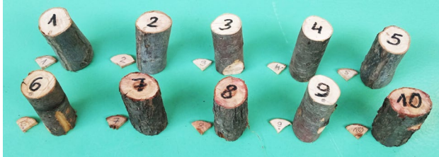
Fig. 12 Samples for testing firewood density and moisture content
