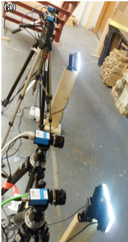
Fig. 3 a Binocular stereo camera systems, b screen shot of the target areas from four cameras.
