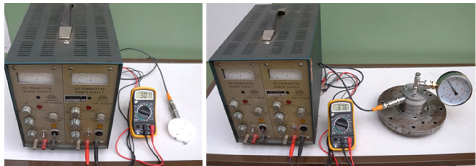
Fig. 8 Set up pressure value in the back -pressure measurement load cell (left) and hydraulic pressure calibration system (right)
