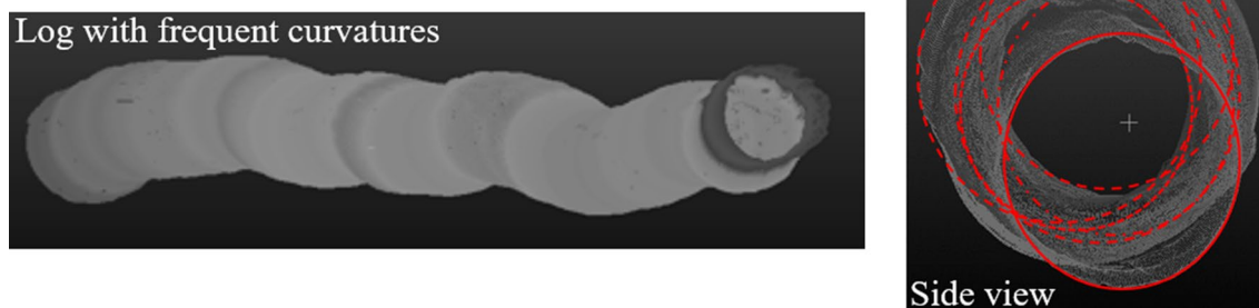
Fig. 2 Frequent curvatures of a beech log (the circles in the side view of this sample should help to follow the curvatures)
