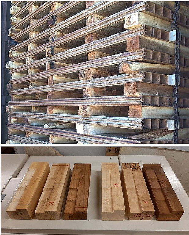
Fig. 1 Above: A set of acacia boards (60×80×1200 mm) after the compression process loaded in the THM treatment kiln. Below: Brinell hardness test specimens of reference and modified acacia and rubberwood. From the left: A, AC, ACT, R, RC, RCT
