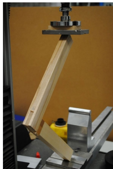
Fig. 4 Compression test on an Instron material tester
