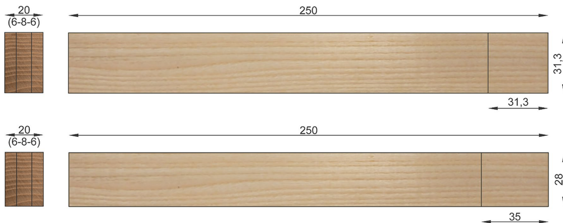
Fig. 1 Dimensions of the test specimen
