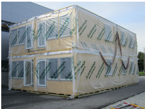
Fig. 13 2 × 2 modules test setup
