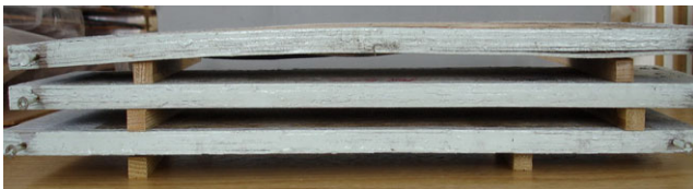
Fig. 4 Delamination and deformation of uncoated plywood panels after 18 months of weathering (from top to bottom: control, NMM-1 treated, mNMM-2 treated)
