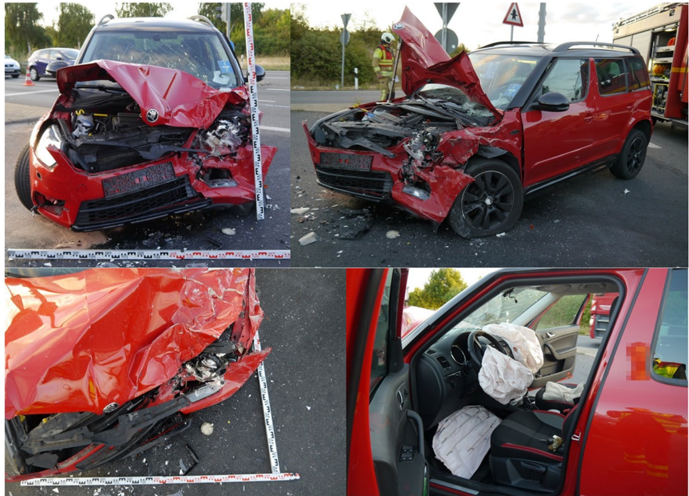
Fig. 1 Exemplary images from the participant survey. Depicted is a crash vehicle, showing the damage pattern, seating position, and airbag status
