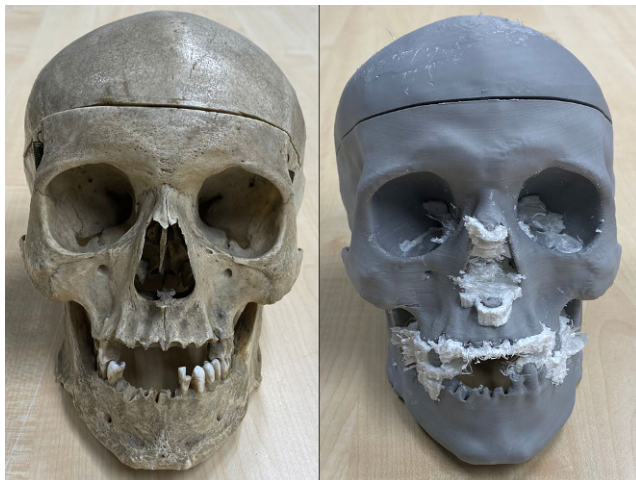
Fig. 1 | 149 Skull specimen (left) and printed model with leftovers from the break away support (right)
