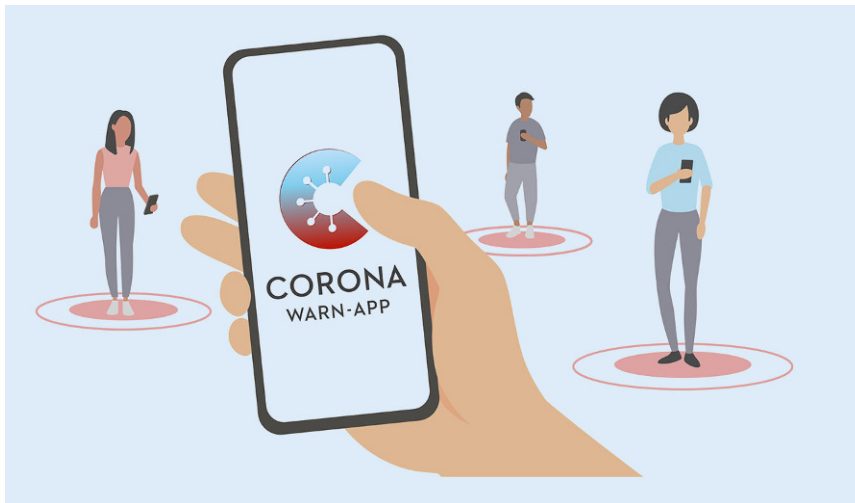
Fig. 1 ▲ Coronavirus warning app. The app is based on a decentralized Bluetooth low-energy technology and informs the user whether he or she has had contact of less than 6 feet for at least 15 min with a person diagnosed with COVID-19. The user remains anonymous at all times. (Adapted from [6])
