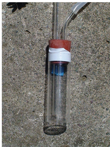
Fig. 3 Instrument used in the experiment investigating wasp behavior. a Tube connected to a funnel for air intake and odorant substances. b Glass or PET tubes to enclose wasps. c : Tube connected to the suction pump
