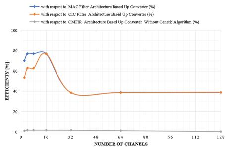
Fig. 6 Register utilization efficiency graph with respect to other structures
