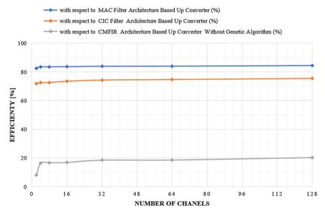
Fig. 8 LUT-flip flop pairs utilization efficiency graph with respect to other structures
