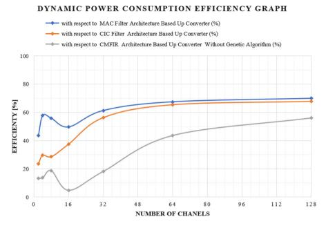
Fig. 4 Dynamic power consumption efficiency graph with respect to other structures
