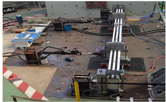
Figure 18 Quasi-static experimental setup on strong-floor
