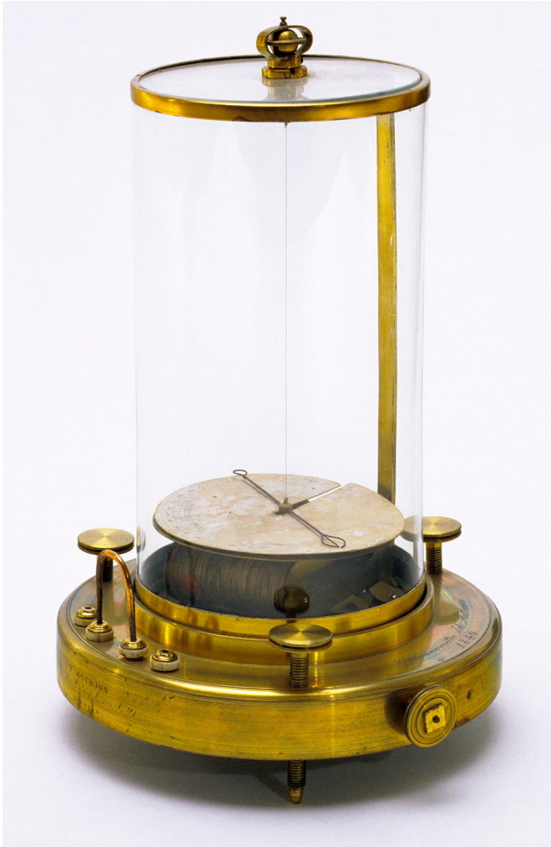
Fig. 7. Astatic galvanometer, Nobili pattern, signed by the Parisian instrument maker T. Gourjon. The brass base ring bears the following engraved words “Matteucci’s Galvanometer / 1840 / Muscular Current.” Using this instrument in 1836 Matteucci studied muscular currents in a frog. Credit: Museo Galileo—Istituto e Museo di Storia della Scienza di Firenze; Teca Digitale ( museogalileo.it )
